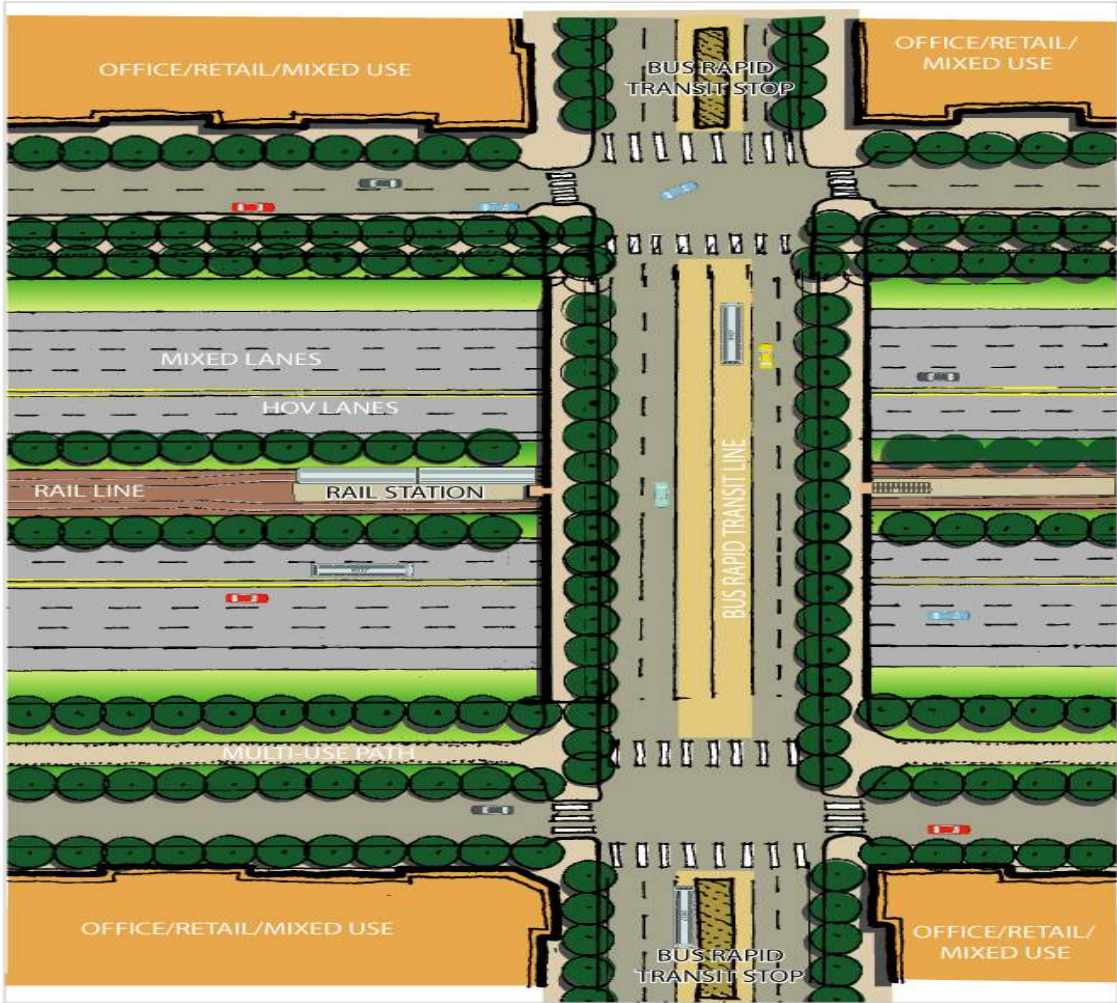
Metro Rural Loop Plan View: Urban Center condition with Transit in middle of the Corridor
